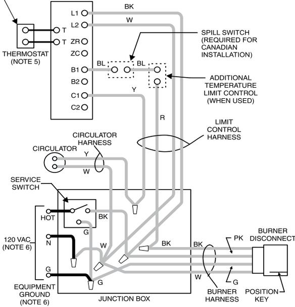
**NOTICE** Burners with Beckett Clean Cut Pump must be used with a primary control that has a valve-on delay (pre-purge). Controls shown have valve on delay (see control manufacturer's instructions for timings.)
