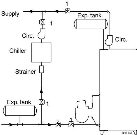
**1** Isolation valve      **2** Balancing valve
