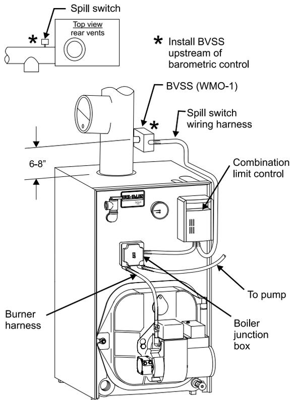
**Figure 19** BVSS wiring diagram
