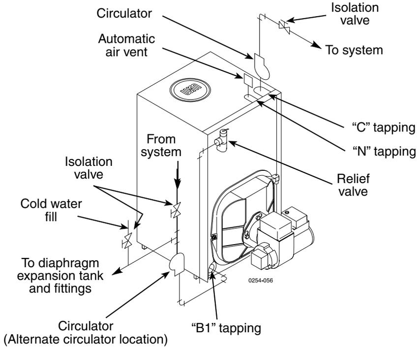
**Figure 10** Piping with CLOSED expansion tank
