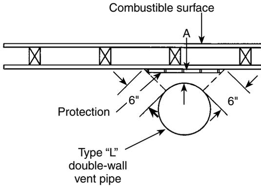
**Figure 25** Back vent clearances
