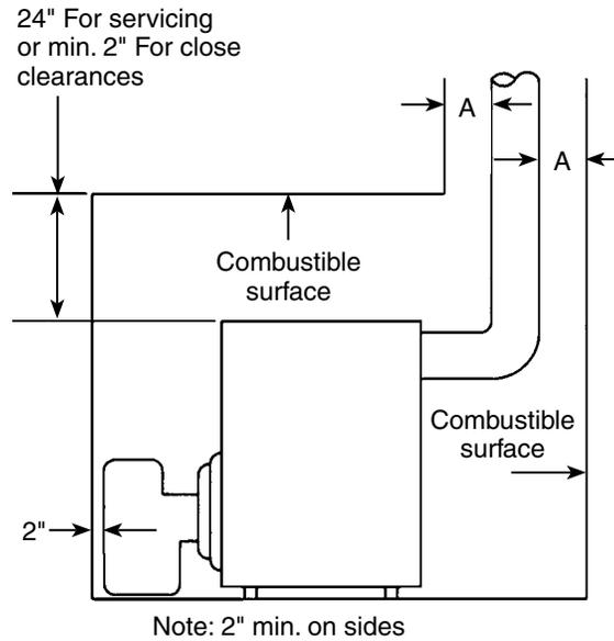
**Table 5** Protection required for clearances less than 6 inches from doublewall vent pipe\*
