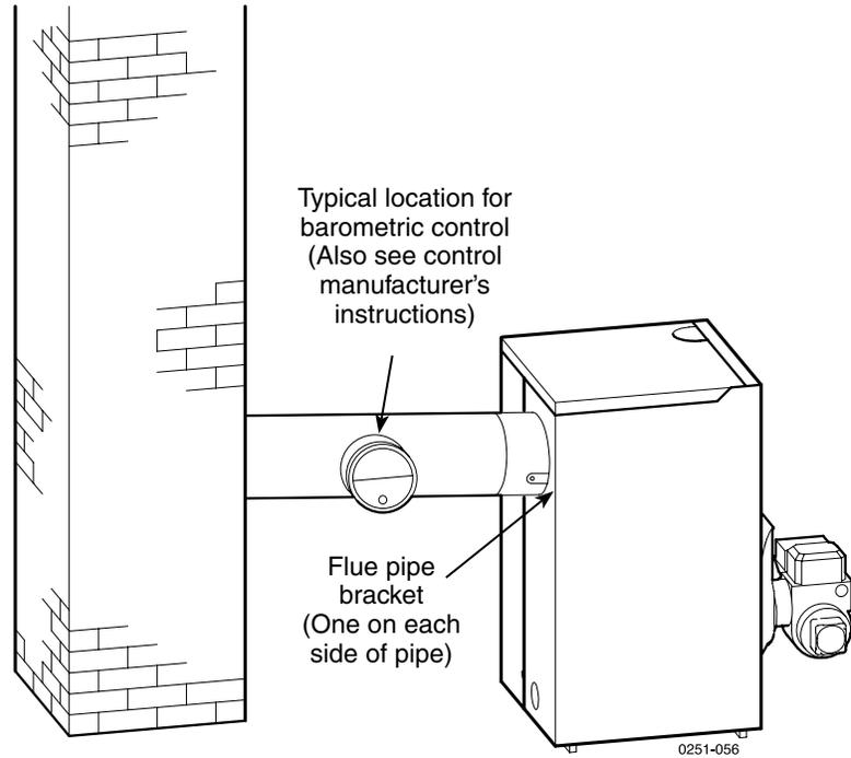
**Figure 8** Top outlet breeching connection
